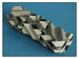
**Figure #1**: GV static mixer with three (3) mixing elements. Each mixing elements has 5 corrugated plate mixing layers stacked at alternating 45° angles relative to the pipe axis. 316 S/S construction with glass-bead blasted finish.
