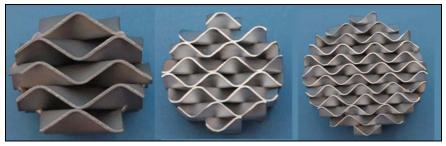
**Figure #5**: The GV mixing element is unique in its ability to "dial-in" the degree of mixing achieved by simply changing the number of mixing layers (corrugated plates) in a specific pipe size. The greater the number of mixing layers (corrugated plates) in a specific diameter, the higher the degree of mixing achieved in a fixed length. The example above shows, from left-to-right, 5 layer, 8 layer and 12 layer mixing elements that fit into the same pipe diameter.
