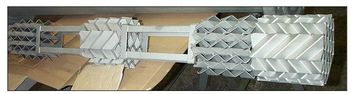
**Figure #7:** The incorporation of spacers between GV mixing elements improves the degree of mixing achieved by taking advantage of the strong turbulent eddies created at the outlet of each mixing element.
