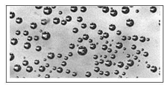
**Figure #4**: The even shear field generated by the GV mixing element assembly creates droplets of consistent size in air-water and immiscible liquid systems and distributes them evenly over the entire pipe cross-section.
