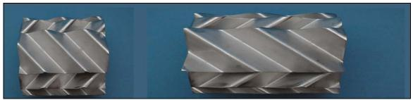
**<u>Figure #6</u>**: The GV mixing element pressure drop can be dramatically reduced by simply changing the corrugated plate angle relative to the pipe axis. Shown at left is the standard GV mixing element (L/D=1.0) with a 45° corrugation angle relative to the pipe axis. At right is the lower pressure drop GV-L mixing element (L/D=1.73) with a 30° corrugation angle.
