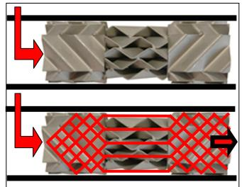
**Figure #3**: Flow pattern through three (3) GV mixing elements of 5 layer construction. Note that adjacent mixing elements are oriented  $90^{\circ}$  relative to each other.
