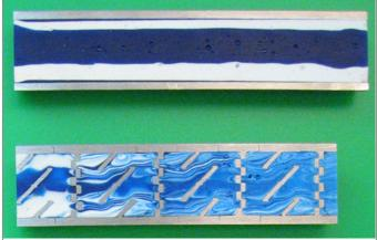
Mixing of blue and white resins in an empty pipe (top) and through a Type GXR static mixer (bottom).
